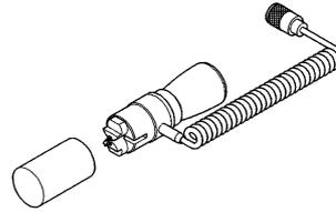
Two needle probe (Cap)
