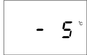
4. The measurement cannot be made because the temperature of the unit is above  $50^{\circ}\text{C}$ . Bring the temperature of the unit down to the operating temperature range ( $0$  to  $40^{\circ}\text{C}$ ), and make the measurement again.
